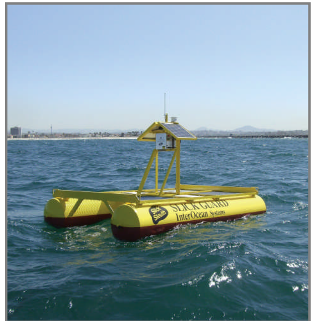
A Slick Guard monitors the water intakes for a desalination plant and a power plant. This system is currently installed in the Middle East.
