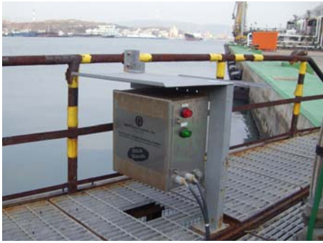
Figure 20. Remote oil spill detection system deployed at tanker terminal for spill monitoring day and night during loading and offloading activities (note loading arm on pier in the background).
