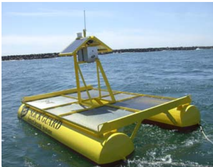
Figures 14 & 15. Catamaran buoy-mounted oil spill sensor for monitoring of desalination plant and power plant intakes. Systems currently installed in Middle East locations. Solar powered with remote telemetry alert.
