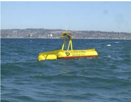
Figures 14 & 15. Catamaran buoy-mounted oil spill sensor for monitoring of desalination plant and power plant intakes. Systems currently installed in Middle East locations. Solar powered with remote telemetry alert.
