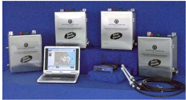
Figure 13. System array supplied through NATO for remote deployment on river flowing into Baku, Azerbaijan region. Wireless alarm/data network communicate to a dedicated base station, for real-time alert via email and text messaging..
