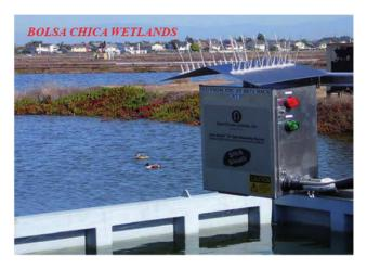
The modem can save this information into files and send it to a remote server over a cellular network provided by Wyless whenever a spill alert occurs, and at fixed time intervals. Going forward, ClearComm can be added to any model Slick Sleuth or add even more functionality to Slick Sleuth as requested by customers.
